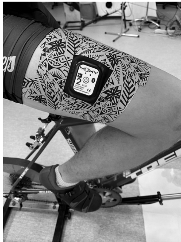
Figure 1. Location of the MOXY monitor on the vastus lateralis muscle belly.
